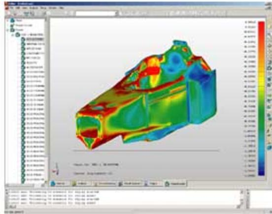
NEiNastran Modeler screenshot showing displacement field from an analysis of the Minardi chassis.
